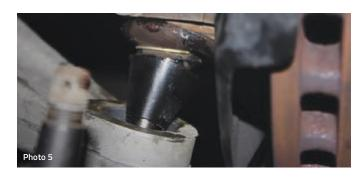
If this occurs, the insert MUST be removed from the old ball joint (without damaging it) and reused. A jaw-type puller such as a tie rod separator works well to apply even pulling pressure. In extreme cases, a bearing separator and hop press can be used. The bearing separator will clamp underneath the insert as the shop press applies pressure on the stud to separate the taper.
